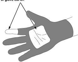
**NOTE:** If gloves are worn, they must be conductive or modified as shown so they do not interfere with operator grounding through the gun.
